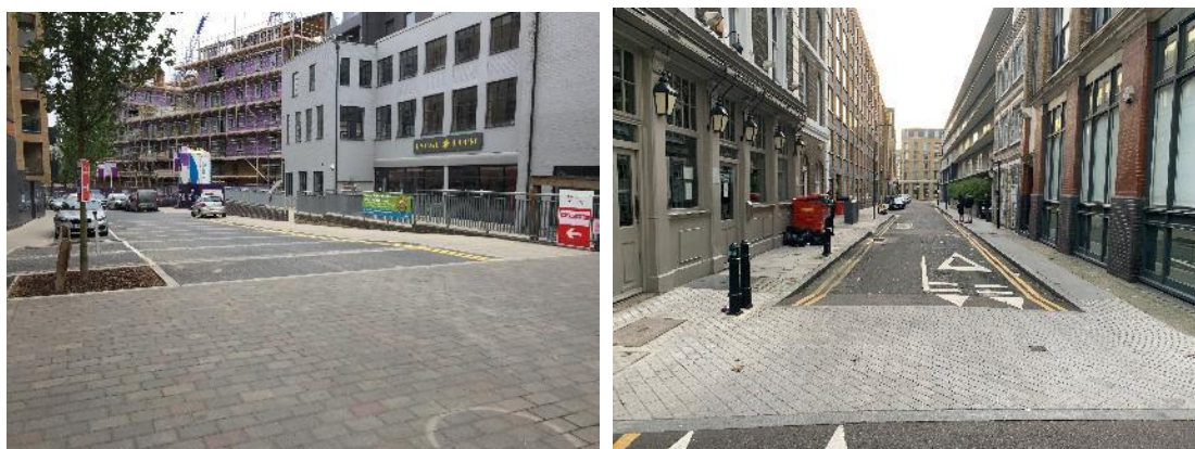
Figure 7-6: Junction crossover treatment (Blackhorse Lane), and Willow Street with recently installed continuous footway (right)
